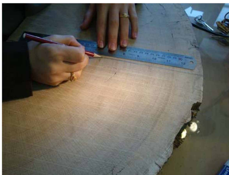
Figure 5. Measuring disc sample tree ring widths in the Golestan research centre lab. using manual measurements (Author, 2010)
